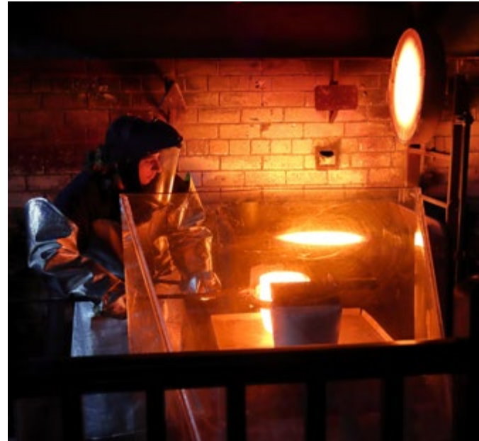
Gold casting at The Perth Mint refinery in Australia.
